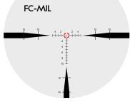
Created and optimized for our low-power variable riflescopes. As first focal plane reticles, elevation and windage markings are valid at every magnification setting, providing precise hold and reference points. The bright daylight center dot is visible under the harshest light. Bold, pointed lines draw the eye to the center of the target.
