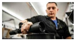
Before they leave the factory, Nightforce riflescopes are subjected to conditions far beyond most anything you will ever encounter in the field. During our impact tests, riflescopes must endure repeated impacts of over 1200 Gs of force on multiple axes.
